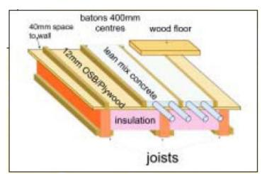
Pipe is laid without joins under the finished floor. All pipe loops return to the manifold, the systems central station. This discreet unit carries the valves that regulate the system. A mixing valve , when on, combines the newly warmed water from your boiler with the return water from the floors to give the gentle, even heat that makes Underfloor Heating so attractive.
