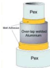
**Flexypipe™'s** low Coefficient of Heat Expansion means it behaves closer to copper or steel than to its plastic counterparts with their large expansion.
