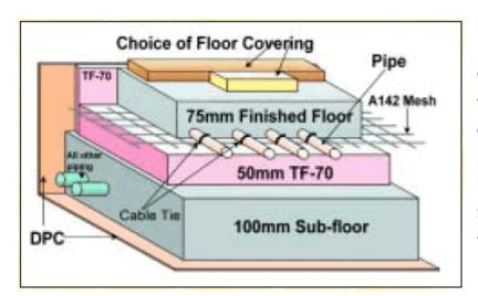
Ground floor is achieved with a 100mm/4" subfloor covered with 50mm/2" of Polyurethane insulation. Pipe is installed on the insulation and covered with a 75mm/3" screed.
